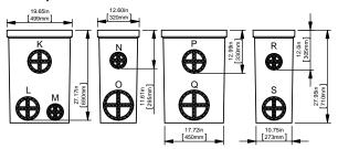
Total capacity of in-line catch basin with 612 base = 27.0 gallons Total capacity of in-line catch basin with 614 base = 36.0 gallons
