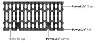
ACO PowerLok® is a patented, boltless locking system. Grates are removed and replaced with minimum time and effort for ease of maintenance. Lugs on the rail opposite the PowerLok® device slots into recesses in the grate. The PowerLok® device is used to engage the lug on the rail at two locations per grate to "lock" the grate to the channel.
