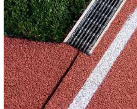
System 4000 is available as a straight channel only. System 2000 radius channels can be used in conjunction with System 4000 open channels if the track requirement is for slotted channels on the curves and grated channels on the straights. 0.5 m channels can be used to create a smoother looking radius. To avoid gaps between channels, miter cut the end. For full details on creating a radius with straight channels, contact ACO.
