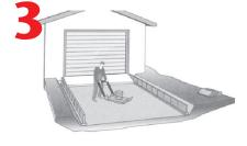
Position PointDrain on a 4" thick concrete slurry bed and ensure it is level.
