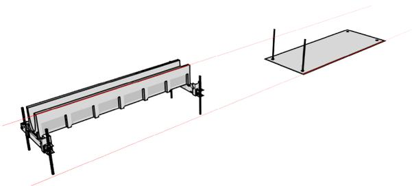
Once the first channel has been replaced, DO NOT lock the adjustable side of the clamp with the wedge yet. This allows some movement of the channel when placing the next channel in line. Do not place the channel all the way to the fixed side of the clamp where it will sit in the locked position. This allows for easier installation of channels.
