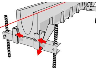
*Note: Ensure the reinforcing bars are installed at least 2 rows ahead prior to installing channels.*
