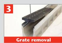
To remove first grate, insert grate removal tool into slots at end of grate, pull up sharply. Remaining grates can be removed by hand.
