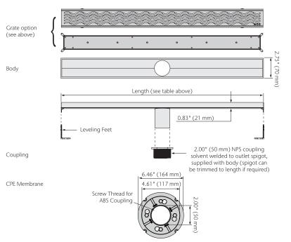
**Note:** Set contains shower channel, grate option, strainer, drain flange coupling, (2) leveling feet, threaded adapter, grate lifting key, and installation instructions
