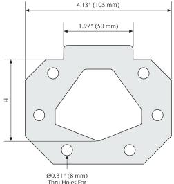
Thru Holes For M6 Connection Bolts
