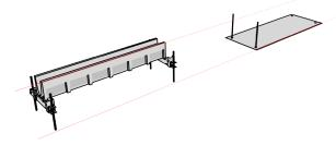
Once the first channel has been replaced, DO NOT lock the adjustable side of the clamp with the wedge yet. This allows some movement of the channel when placing the next channel in line. Do not place the channel all the way to the fixed side of the clamp where it will sit in the locked position. This allows for easier installation of channels.
